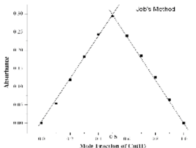
Fig. 7 : Job's method of continuous variation: [concentration of Cu(II) = 2-HAPSH] = 1.0 mL of 1.0 \times 10^{-4} M, pH = 6.0 and \lambda_{\text{max}} = 380 \text{ nm}
